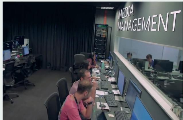
In the news area, a fully redundant KVM system comprising two Draco tera 160 port enterprise switches, and redundant variant CPU and CON units provides totally reliable and secure connectivity to a wide range of broadcast equipment using a mixture of DVI, DisplayPort, serial, analog audio and USB data transfer.
