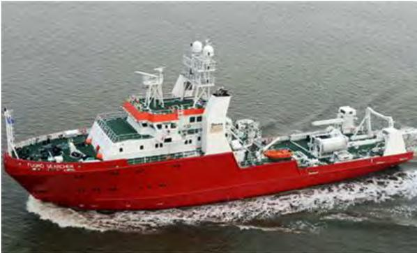
The 65 meter MV Fugro Searcher is a new, highly equipped geophysical survey vessel providing an acoustically quiet and stable platform for operation in the North Sea and International waters. The vessel is equipped with an array of echo sounders, sonar equipment and sea-bed profilers to service the offshore oil and gas and cable engineering industries.
